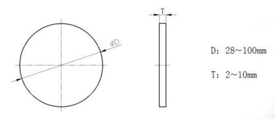
Material: Carbide Substrates For PDC can be supplied matching materials according to customer's need.
