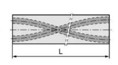
Rods with Two Straight Coolant Holes
